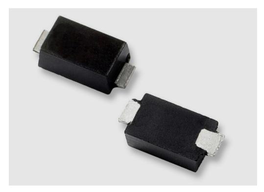
The SZSMF4L from Littelfuse are transient voltage suppression diodes supplied in a compact SOD-123FL package that provides greater design flexibility and occupies less space than previous technologies. The footprint is just 3.85 mm by 2.35 mm. In addition to being AEC-Q101 qualified, the SZSMF4L series meets ESD Class 3 and IEC 61000-4-2 certification standards.
